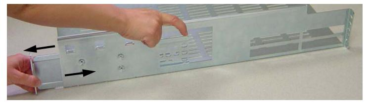
Figure 2-2: Separate the Sliding Bracket From Both Sides of the Shelf Unit
